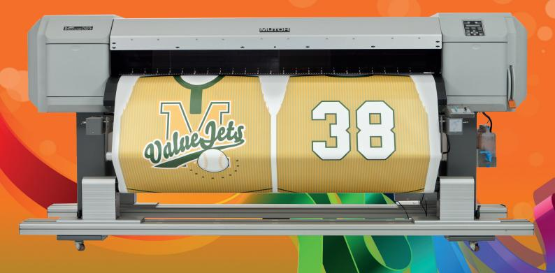
Transfer sublimation printing up to 1625 mm (63.97") Staggered dual head setup with latest generation 1440 nozzle piezo heads Production speeds between 42 & 65 m²/h Mutoh water-based disperse dye inks Ideal for production of soft signage, sportswear, gadgets, ... Environmentally friendly printing - high level of operator safety
